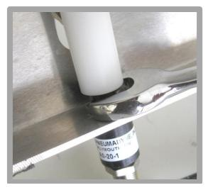
3. Using a 9/16" Wrench, remove the hex nut and star washer from the Air Valve.
