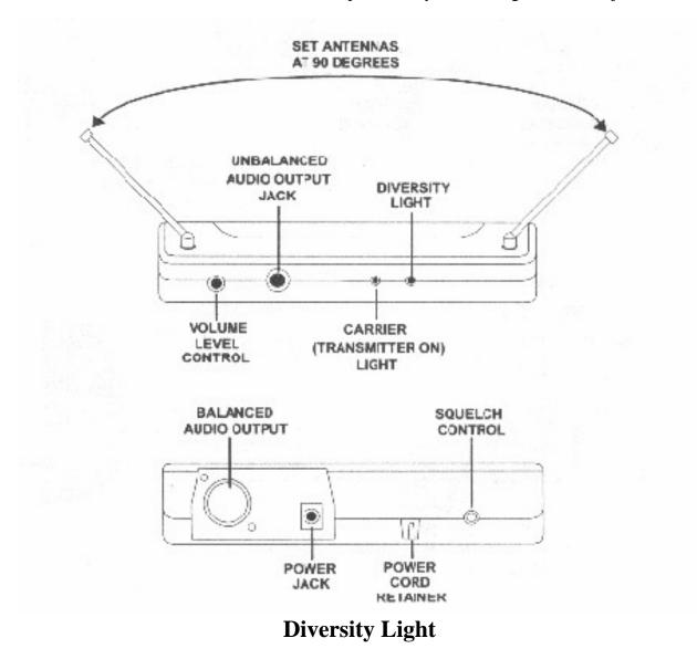
The diversity light is a bi-color LED (orange/green) that is illuminated any time the receiver has power. When it changes color this indicates that the diversity circuit is activated to optimize reception.
