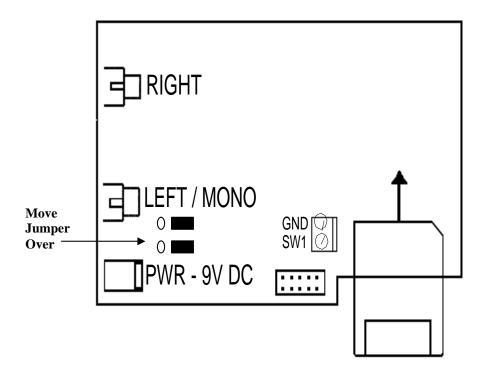
In the event your ribbon cable becomes damaged, broken or shorted, disconnect or unplug the ribbon cable. Ensure that the 22 gauge red and black wires are properly connected to "GND" and "SW1". Plug in the 9V DC – 12V DC power supply and ensure that the phono/RCA cable is plugged into either "RIGHT" or "LEFT" female phono jack.
