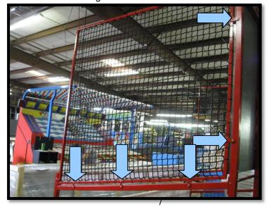
Using the supplied wire tie supports and rope, you can choose whether or not to install the canvas bottom. Simply secure the canvas to the canvas rods using the wire ties. Run them through the eye-lets and then wrap the rope around the canvas rod and into each eye-let.
