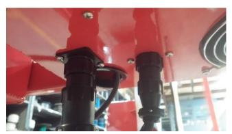
Input Plugs located on the bottom of the Sound Unit Control Box:
