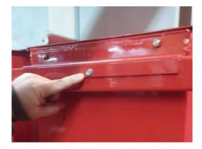
12. Attach the Game Clock Display Box from Support Beam #3 using provided nuts, washers, and bolts.
