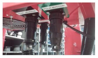
Input Plugs located on the bottom of the Electronics Assembly Box:
