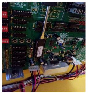
4. After you have the old programmed IC out, gently insert the new programmed IC into the slot. Make sure you line up the pins with the socket. Also notice there is a knotch on the programmed IC as well as the IC socket. These knotches need to line up.
